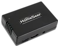
1. Unpack the HomeTroller Pi Hub and AC power supply. Connect an Ethernet cable to the unit and attach that to your router or network switch.
